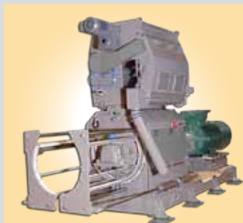
Hammermill with automatic change of screens during operation
