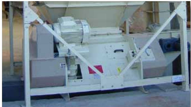
Crumbler beneath cooler
