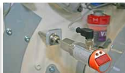
Temperature gauge on grinding chamber
