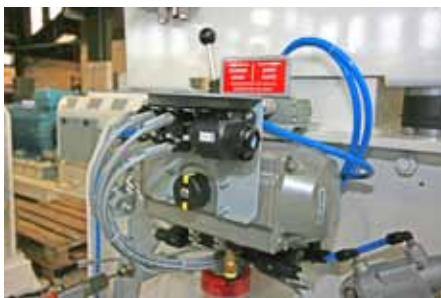
Splitter box for a quick connection to the supervision
