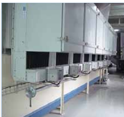
2 - way cooler fitted with filters
