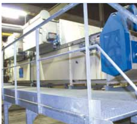
2 - way cooler fitted with filters
