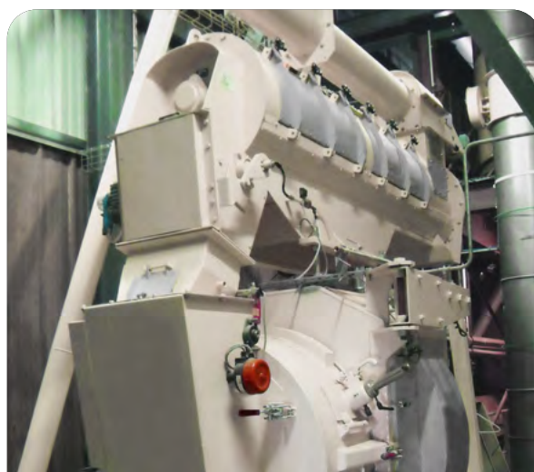
Long life horizontal mixer conditioner on pellet mill
