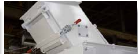
Magnet plate on feed chute
