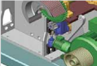
Slow rotation by gearmotor
