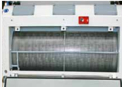
Grinding chamber fully taken up by the screens
