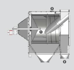
The cleaning of coarse wastes is obtained by the flow of good products into a drum • through the mesh of a rotary cylindrical screen.
